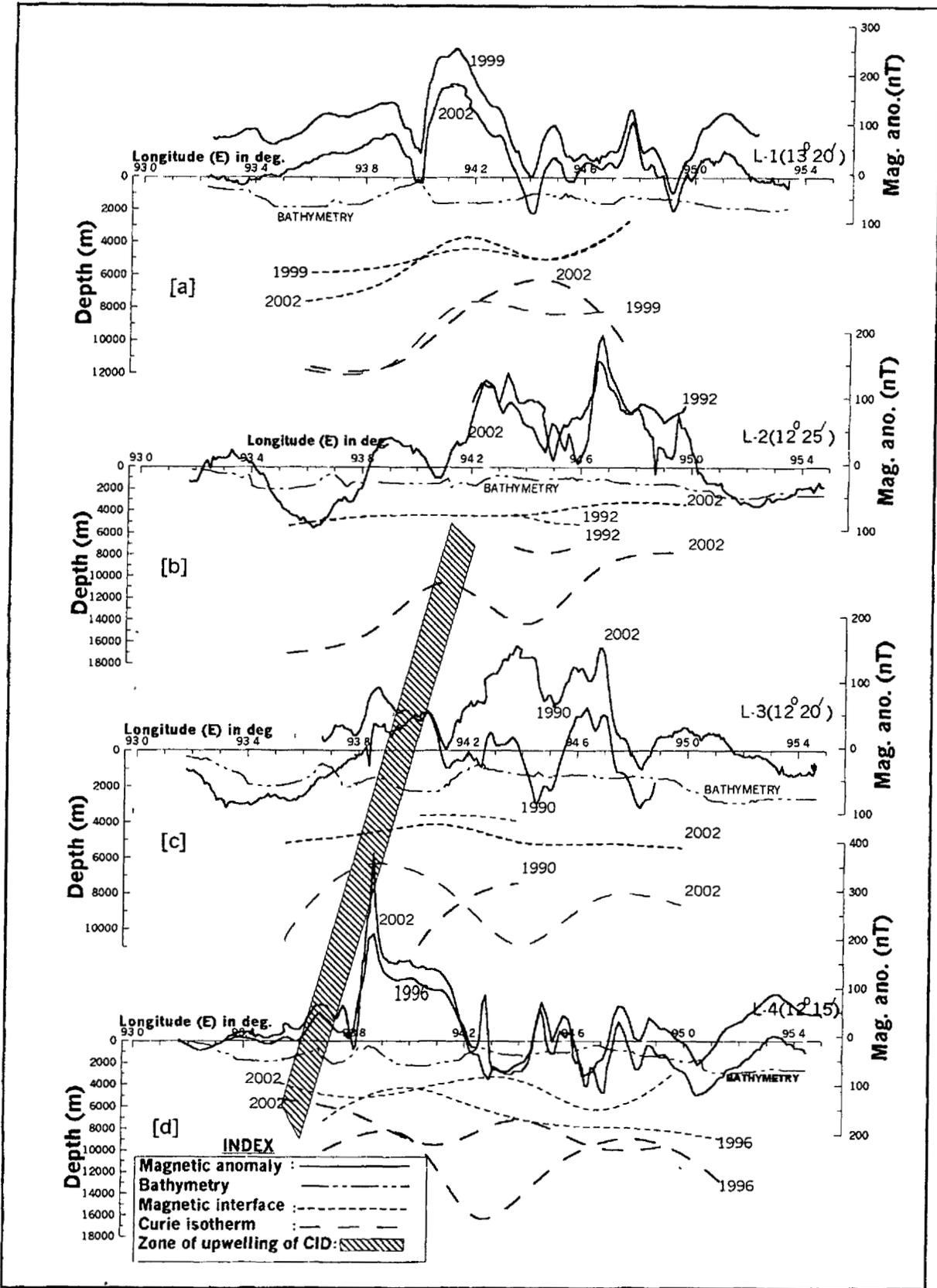
Fig.2. Magnetic (TF) anomalies along the four traverses around Barren and Narcondam island and the changes in geoisotherms since 1990
